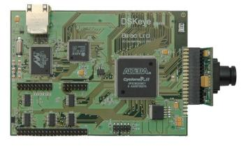
The DSKeye from BiTEC Ltd is a TI DSK daughterboard gathering the latest FPGA technology, a 5.2 mega pixel camera and user configurable interface options to deliver a Smart Camera system for development and research at a fraction of the cost normally associated with such technology.
